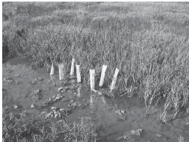
FIG. 2. Photograph of mylar caps sealing sediment cores (containing S. foliosa plants and rhizosphere sediments) being incubated in situ during isotopic enrichment (Experiment 4). Caps are ~30 cm high. Photo credit: S. M. Moseman-Valtierra.
