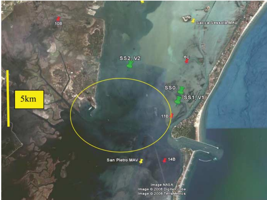
Figure 7. Sediments from area SS0 were used to build banks V1 and V2 in areas SS1 and SS2.
